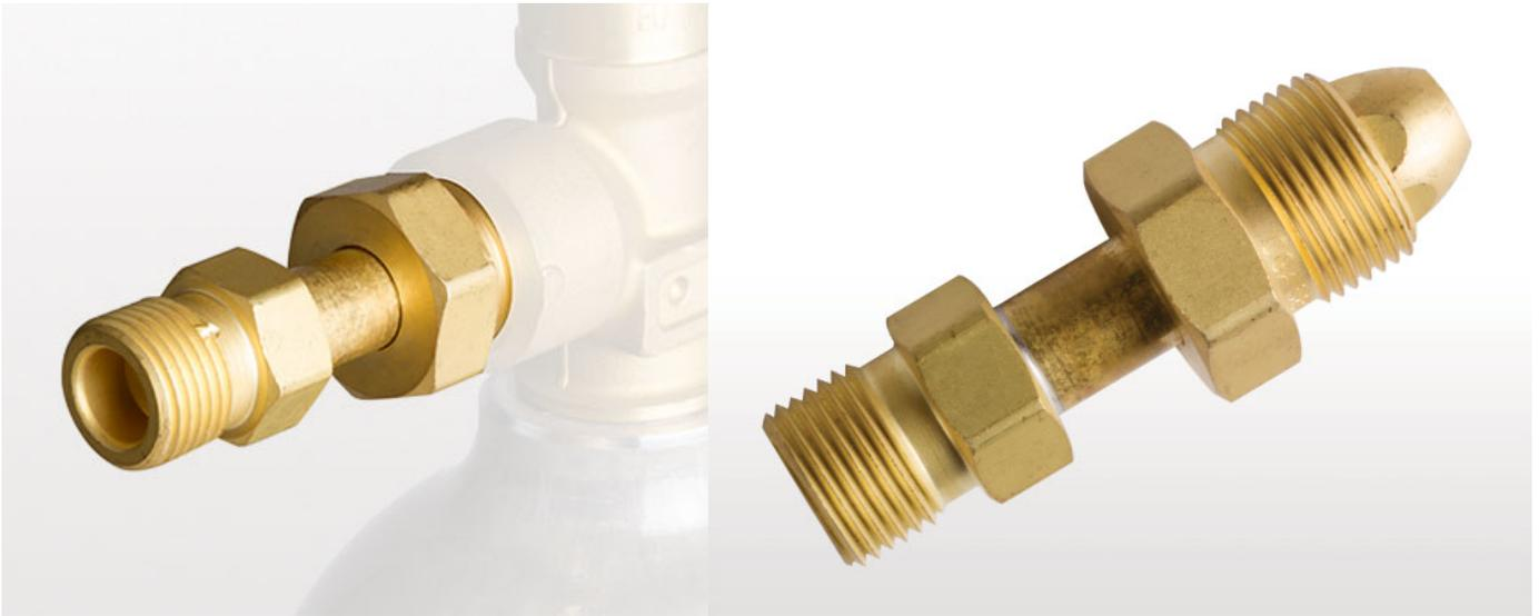
Adapter fitting quickly converts Nitrogen CGA 580 cylinder to compressed air CGA 346 for filling with compressed air. Cylinders are to be filled to 2000 psi on a 2216 psi filling system with Nitrogen or compressed air.
